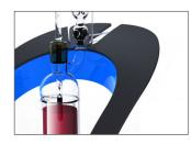
» Fill boiler to the line and turn on heat
